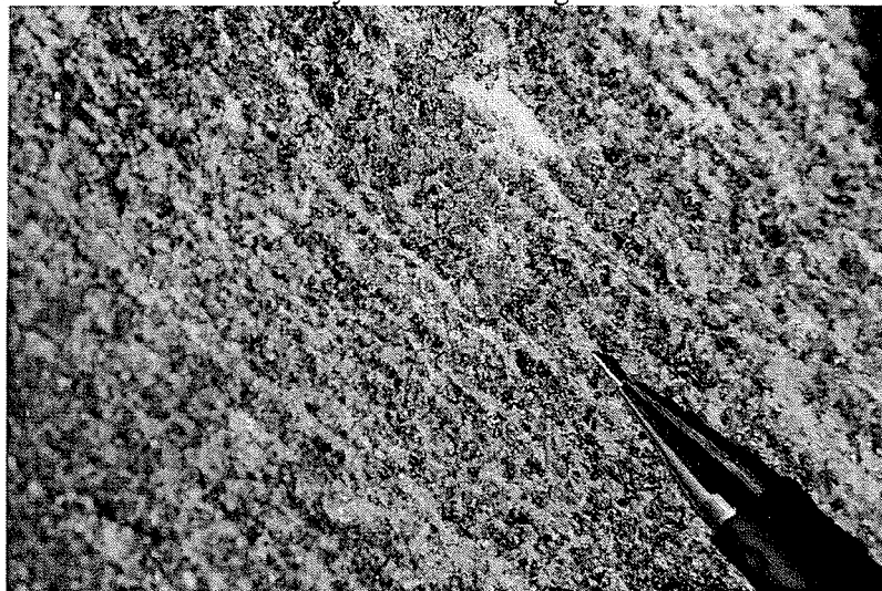
Figure 2-2. Diopside-feldspar gneiss. Dark grains are diopside, light grains are potassium feldspar and quartz.
