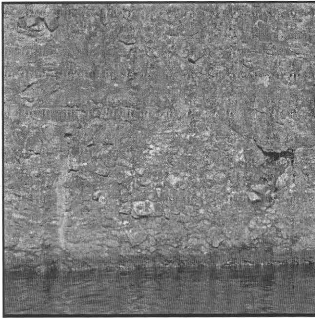
Figure 27. Fault Breccia Observed Along East Bank of Kyser Lake (south of the Dolgeville dam).
