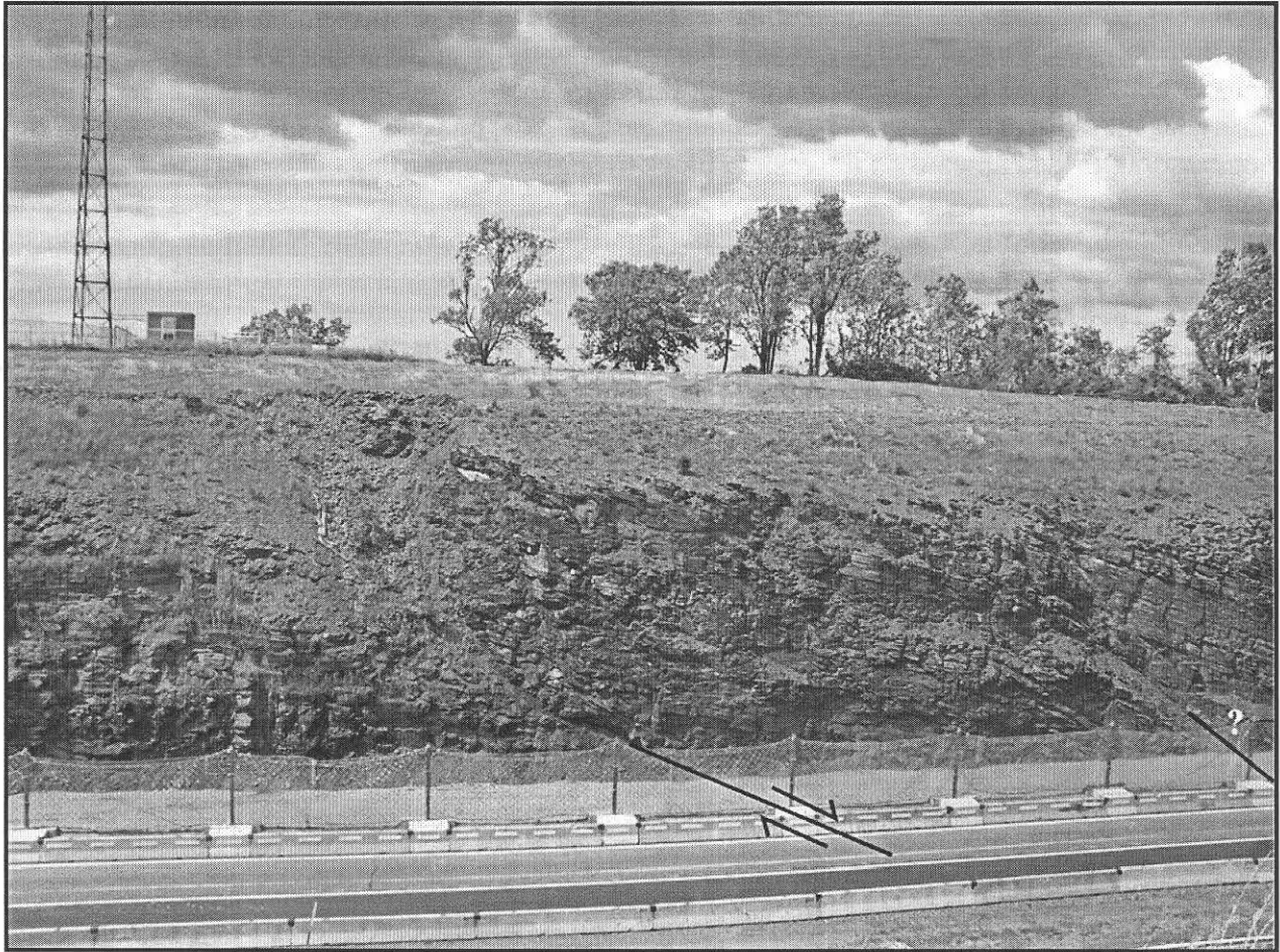
Figure 35. Little Falls Fault “C” at the Thruway Cut (photo looks NNE). Offset is down to the east, juxtaposing Dolgeville Formation and lowermost Indian Castle Member (west block) with Indian Castle Member. A minor splay can be seen on the right with an unknown offset within the black shales.
