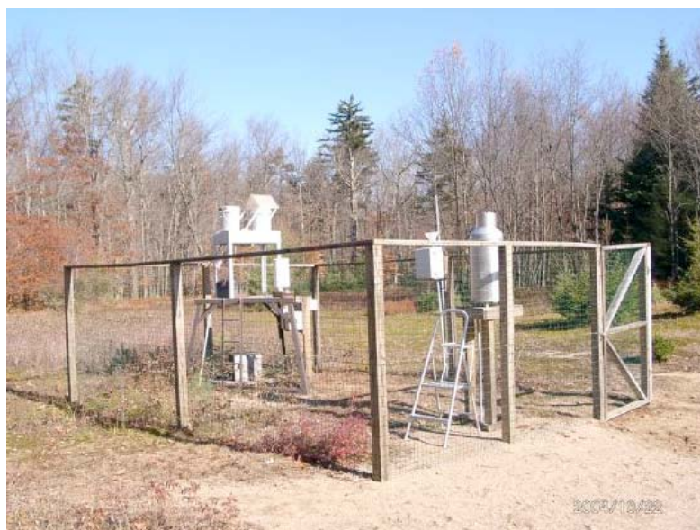
Figure 7: NADP site NY29 at Moss Lake showing wet/dry collector, rain gage and other meteorological equipment (from http://nadp.sws.uiuc.edu/sites/siteinfo.asp?net=NTN&id=NY29 ).
