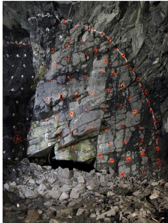
Figure 14 - Geological map and southward view digital image of west slash of North Cavern below 85th street in NYC. Note the internal structure dominated by internally sheared gentle SE-plunging isoclinal recumbent folds of early SE-dipping gently inclined foliation in Hartland formation (O€h). Recrystallization during folding and shearing produced penetrative mica foliation (Feature 13.) that formed parallel to transposed compositional layering. Gently inclined foliation joints are prominent discontinuities (J 1 ) and have formed parallel to the foliation and parallel compositional layering. These are intersected by steep NNE-trending (J 2 ) and NW-trending (J 3 ) joints and faults producing overbreak (light green shading). (Digital image taken 19 December 2012.)
