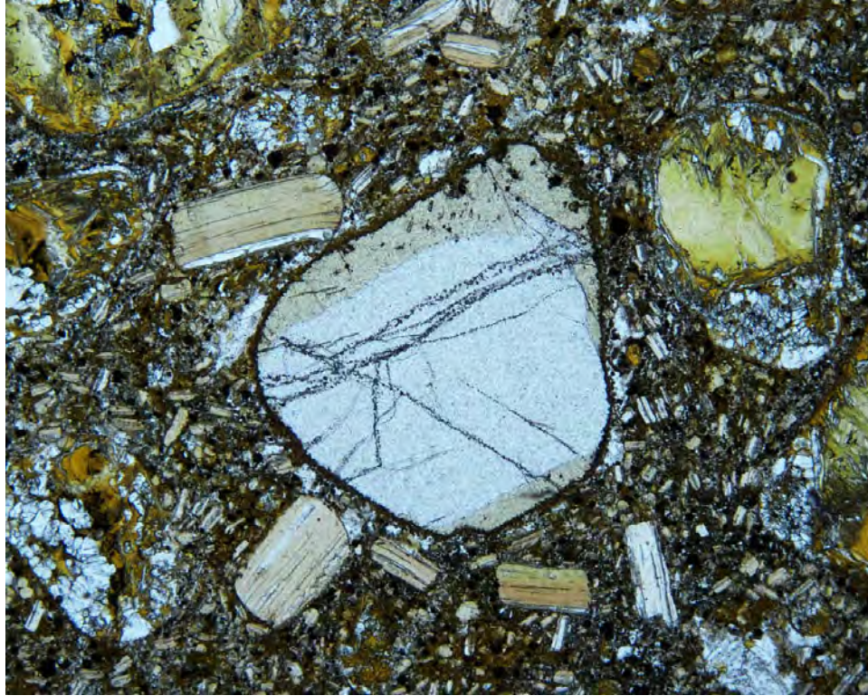
Figure 8. Clinopyroxene, phlogopite, and serpentinized olivine macrocrysts in the Six Mile Creek kimberlite (sample SMC-2A, PPL).
